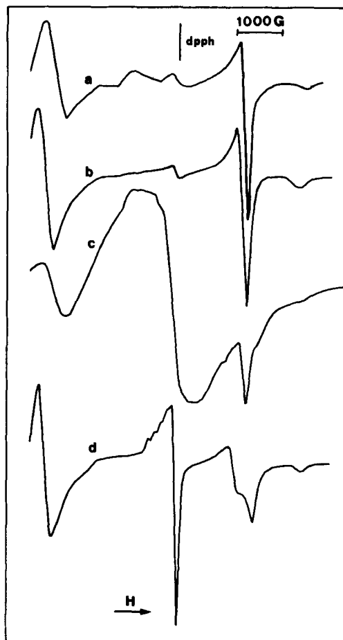
FIGURE 1 X-band ESR spectra recorded on polycrystalline samples of (a): \text{Cu}(\text{L}^1)_2 \cdot 2 \text{CH}_3\text{OH} (at 123 K); (b): \text{Cu}(\text{L}^4)_2 \cdot 1.5 \text{H}_2\text{O} (at 298 K); (c): \text{Cu}(\text{L}^3)_2 (at 298 K); (d): \text{Cu}(\text{L}^3)_2 (at 123 K).
